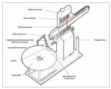
Annotated diagram of HAESL SRMS showing direction of axis-travel
