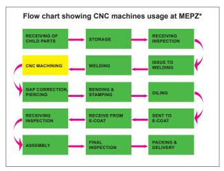
The above chart shows the role of CNC machines. The child parts are collected in the beginning followed by the welding process. After welding, the entire work is done by CNC machines. \*SAF has a unit at Madras Export Processing Zone (MEPZ), Chennai
