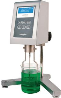
speed, selected spindle, viscosity, percentage torque, shear rate, and shear stress on the 5-line display. Enter the sample density, and the unit calculates and displays kinematic viscosity (cSt) as well.
