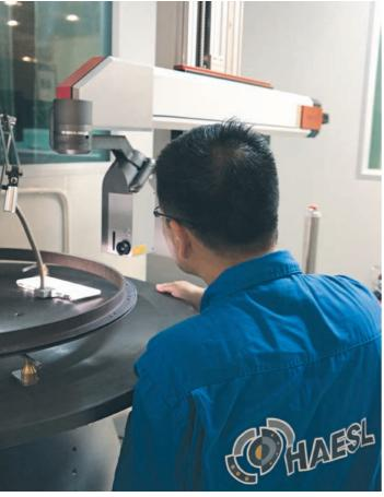
HAESL employee using SRMS (Seal Ring Measurement System)
