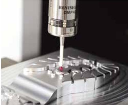
OMP40-2 machine tool probe
