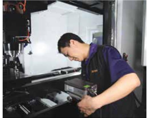
Hartford employee using XL-80 laser interferometer for machine calibration
