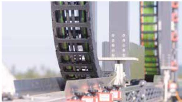
IT REDUCES THE DE-ICING TIME TO SEVEN MINUTES AND THE WASHING TIME TO TWENTY MINUTES. THE SYSTEM CONSISTS OF THREE BEAMS, ATTACHED TO EACH OF WHICH ARE TWO TELESCOPIC ARMS AND BARS. THERE IS A NOZZLE SYSTEM IN THE BARS AND ON THE FLOOR.
