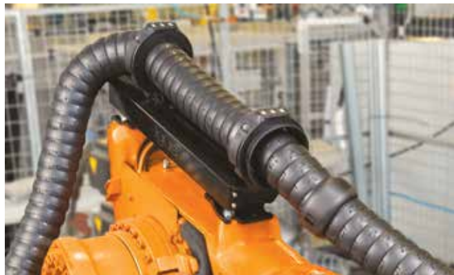
Cost-effective and safe: The new TR.RSEL retraction system with energy chains ensures trouble-free operation of robots. (Source: igus GmbH)
