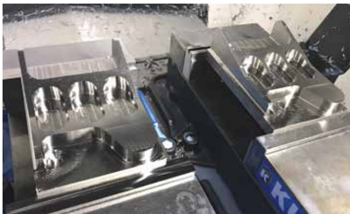
In the Okuma demonstration, the VERICUT Force Optimized finished part on the left was produced more than 20 percent faster than the original programmed part on the right.
