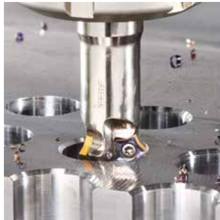
Fig 4: CHAMFMILL cutter with 5 point star insert
