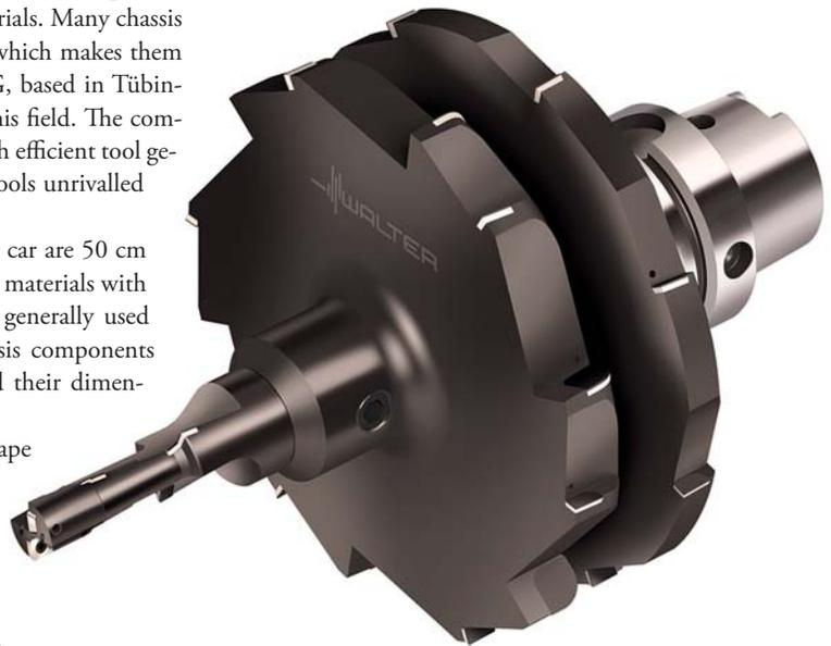
Simultaneous face milling of the upper and lower sides on the upper connection of a drag bearing. Then a stepped hole is drilled into the connection, without changing tool, and the rear side is deburred circularly. Image: Walter AG
