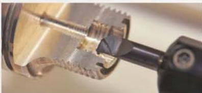
**microscope** Micro Tools for Small Bores
