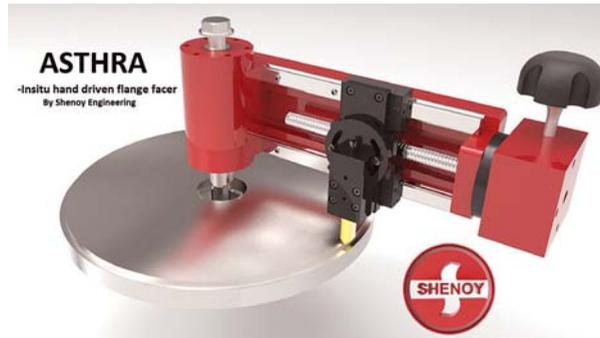
Ø 1” to Ø 6”. The main components of this facer, like arm, housing, is cast from Aluminium to make it light. Sliding surface is made of LM guides and blocks to provide utmost frictionless smooth movement, keeping in mind the operator’s fatigue. The tool is moved over the LM guides through a leadscrew-box nut arrangement,
