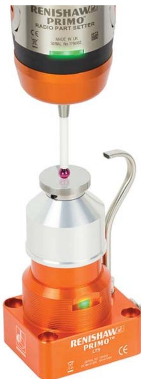
Global engineering technologies company Renishaw has launched the Primo™ LTS (length tool setter) at CIMT, Beijing, China. The Primo LTS is a single-axis tool setter which allows users to set tool length, check for breakage, and compensate for thermal growth on a CNC machining centre.
