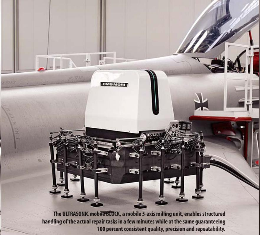
The ULTRASONIC mobileBLOCK, a mobile 5-axis milling unit, enables structured handling of the actual repair tasks in a few minutes while at the same guaranteeing 100 percent consistent quality, precision and repeatability.
