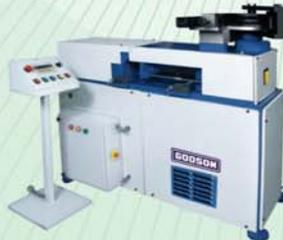
HYDRAULIC PIPE & TUBE BENDING M/c.
