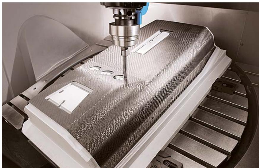
The ULTRASONIC 260 and ULTRASONIC 360 offer 5-axis-machining and profit from the rigidity, long-term stability and thermo-symmetric concept of the machine that ensures a high level of precision in continuous operation.
