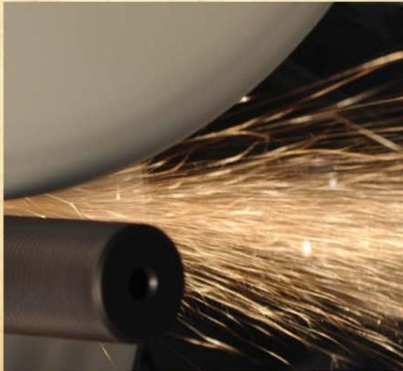
Uncontrolled heat build up can lead to discoloured and damaged components
