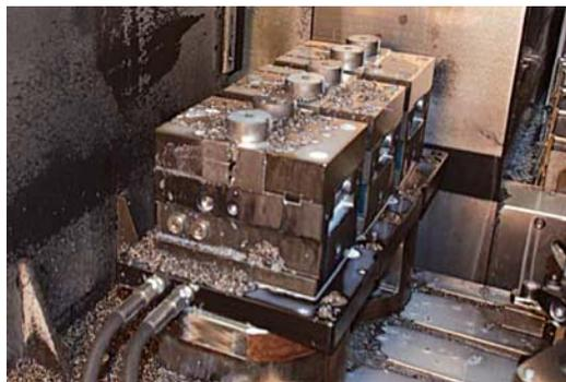
base body in order to maintain a secure reference. However, the moveable jaw is guided by interior slides at the base of the vice to avoid upward movement of the work-piece. The vices are totally hermetic and thus no cleaning operations are needed.
