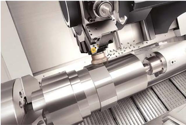
The new NLX 6000|2000 manages the whole range of high-performance turning in the field of long parts with large diametres from 2-axes turning to 6-side complete machining
