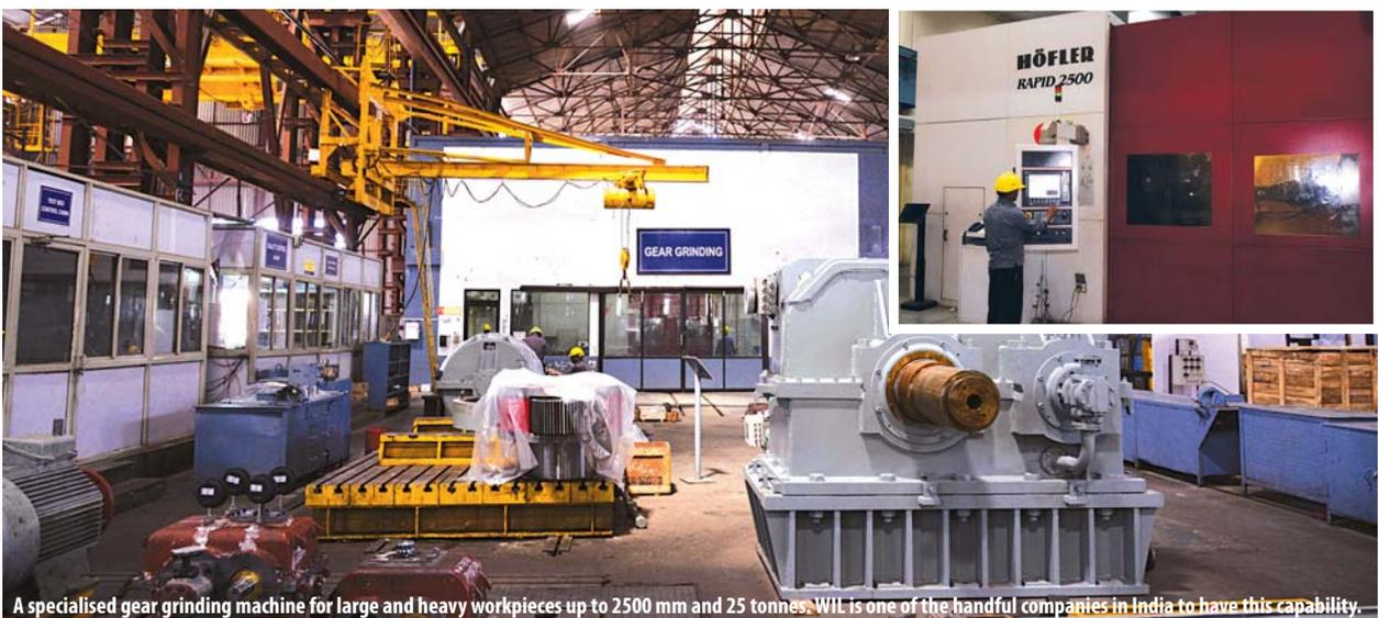
A specialised gear grinding machine for large and heavy workpieces up to 2500 mm and 25 tonnes. WIL is one of the handful companies in India to have this capability.
