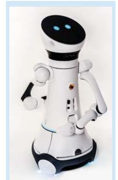
The modular design of Care-O-bot 4 allows the set-up of an individual robot platform for various applications, decisively reducing the costs for developing new service robotics solutions. Source: Fraunhofer IPA, Photo: Rainer Bez
