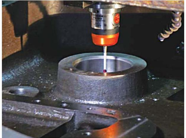
Amazing 90% reduction in inspection cycle time on turbocharger housing
