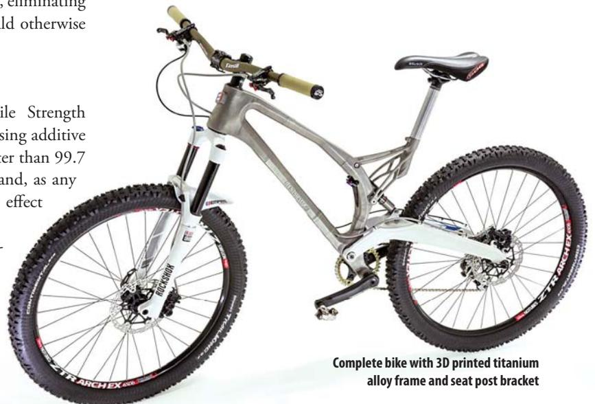
Complete bike with 3D printed titanium alloy frame and seat post bracket
