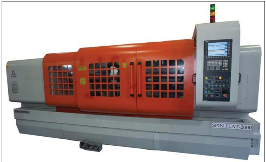
The space availability in the machine allows the operator to load and unload heavy components using overhead cranes. The turret is mounted towards the non-operator side ensuring clear visibility and access.
