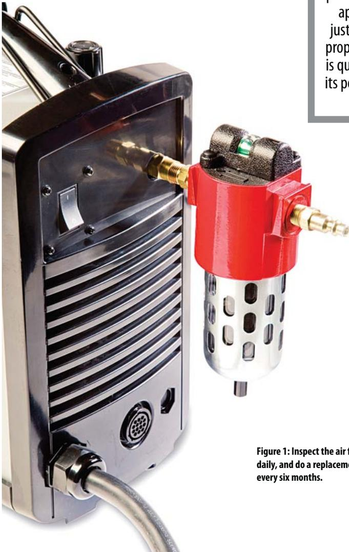
Figure 1: Inspect the air filter daily, and do a replacement every six months.
