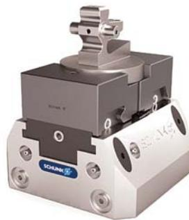
**The jaw quick-change system BWM minimizes the set-up time of the TANDEM KSP plus clamping force blocks to less than 30 seconds.**
