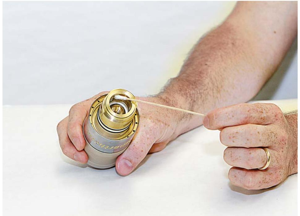
Figure 2: A cotton swab can be used to clean hard to reach areas
