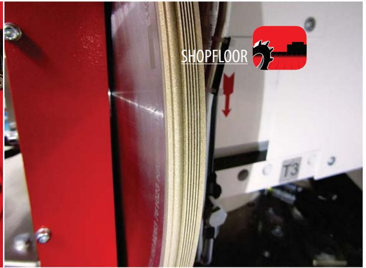
Example of an MD25 grinding wheel Ø400 mm, complex profile dressed with WireDress
