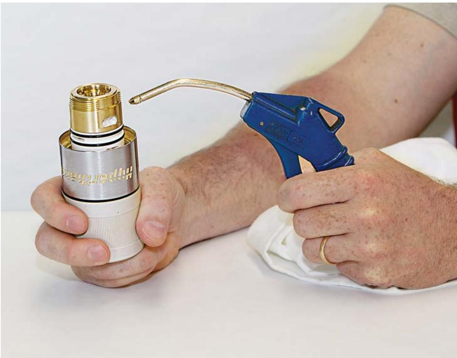
**Figure 3: Clean the inside of your power supply by blowing out contaminants**
