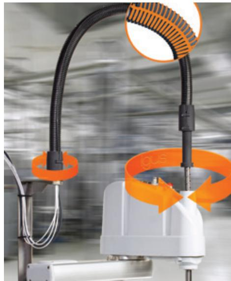
and the fixed end, as well as the corrugated hose with the e-rib. The special feature lies in the new rotary connection, which absorbs the torsional forces. Here, integrated ball bearings ensure a smooth-running energy supply system that is resistant even to high accelerations. The corrugated hose is reinforced with an e-rib so that it can only move in one spatial direction. The guide elements on the sides give the hose unsupported length.
