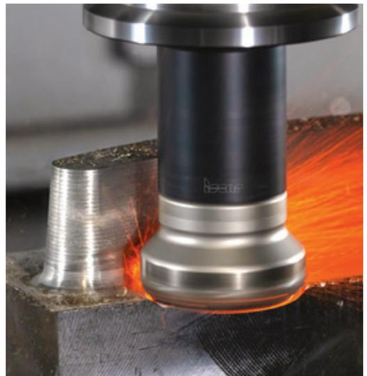
**Fig. 3 – Milling cutters with indexable round inserts from ceramics provide considerably increased cutting speeds for higher productivity.**
