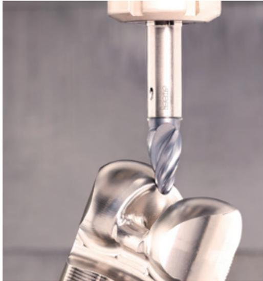
**Fig. 2 – Machining a femoral knee implant component with a MULTI-MASTER endmill and exchangeable taper barrel head.**
