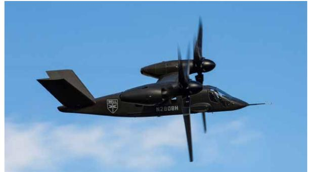
In parallel to the demonstrator program, the GKN Aerospace global design team continues to work with Bell to optimize the V-Tail design to meet customer requirements for the FLRAA program. The two compression-moulded Access Panels have been manufactured from recycled thermoplastic waste material from the two Ruddervators.
