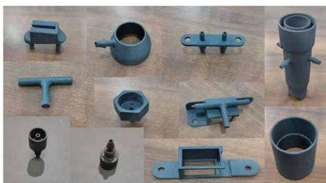
it would have taken 4-5 months to manufacture these quantities using the conventional process. With HP 3D printing technology, these parts were printed in just 24 days. AgVa Healthcare's ventilator is an ICU ventilator with Volume, Pressure & Flow Control. The entire system can be controlled by a capacitive multi-touch interface without the need of compressed medical air. It is extremely portable and can be used in ICU transport or homecare.
