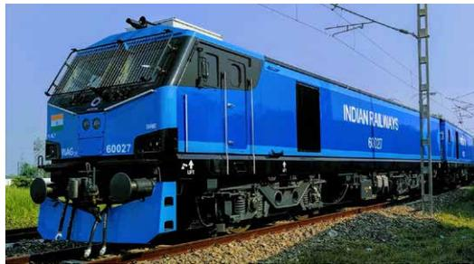
trains in India by at least 20-25 kmph. Equipped with Insulated Gate Bipolar Transistors (IGBT) based propulsion technology, it would lead to considerable savings in energy consumption due to use
