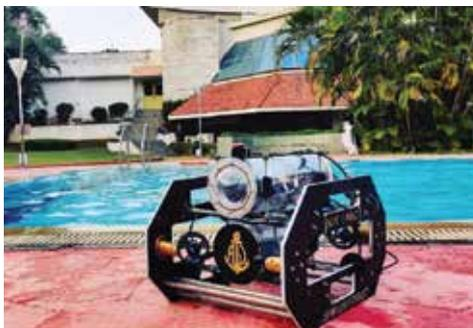
AUV is currently capable of carrying out navigational and other tasks pre-fed into its memory with good precision and near-zero error. Weighing 19.6 Kgs, MEC's Black Pearl is a fully autonomous operation and carries power onboard through a Lithium Polymer Battery.
