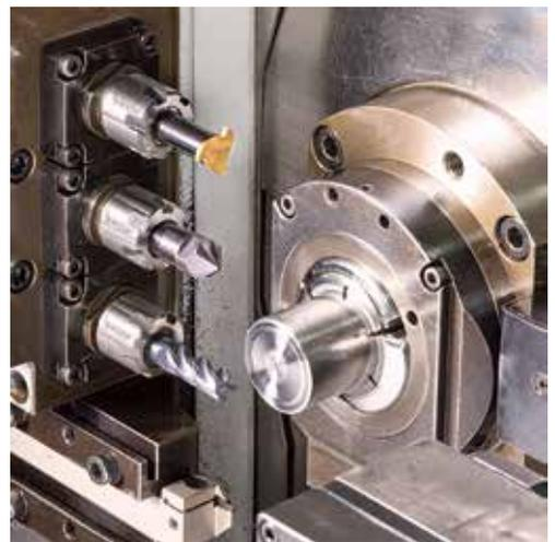
Figure 4: MULTI-MASTER Tools in multifunction machine tool post
