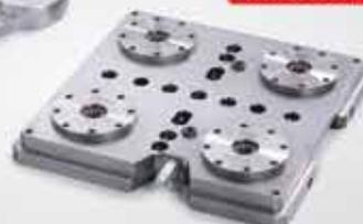
Clamping and locating repeatability less than 0.005mm
