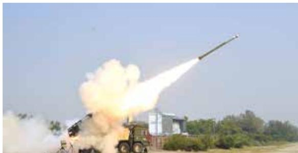
seconds interval between two firings. Both the missiles were fired to engage a target located at 20-kilometre range and high accuracy was achieved. The missile was integrated with live warhead with proximity fuse and was tracked by multiple range systems viz. telemetry, radars, Electro-Optical Tracking System (EOTS), which confirmed the text book flight performance.
