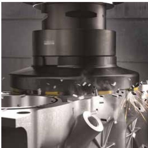
A range of thermal and mechanical properties makes for challenging machining when it comes to bi-metal materials. Existing milling cutters for this application are complex and require adjusting, resulting in compromised throughput rates.
