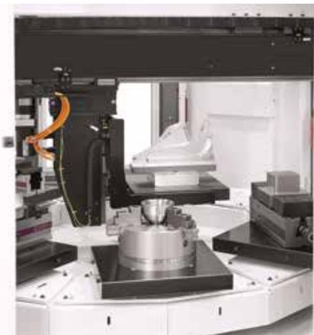
THE AUTOMATION SOLUTION'S HANDLING SYSTEM GUIDES ONE RAW PART AFTER ANOTHER TO THE MACHINE CENTER AND REMOVES THE MACHINED WORKPIECES TOGETHER WITH THE PALLET AFTER THE CUTTING PROCESS HAS BEEN SUCCESSFUL."
