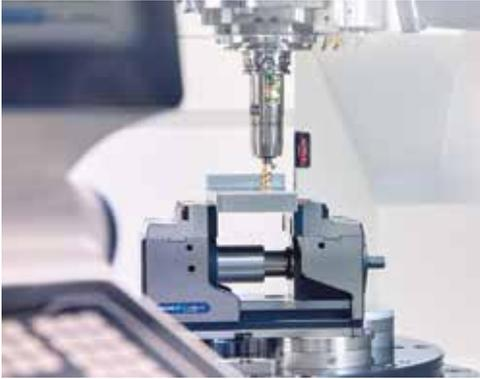
Vibrations, chatter marks, tool failure – what has so far robbed many a machine operator of sleep will soon be a thing of the past: With the smart iTENDO hydraulic expansion toolholder, SCHUNK and start-up company TOOL IT present the world's first intelligent toolholder that monitors the machining process directly at the tool, and allows real-time control of the cutting parameters.
