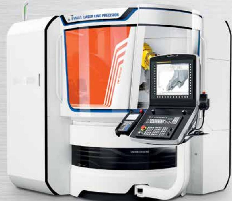
The LASER LINE PRECISION replaces previous methods for grinding and eroding ultra-hard materials, such as PCO, CVD-D, CBN and MCD through the use of lasers. It holds rotation symmetrical tools of up to 200 mm diameter and up to 250 mm length as well as indexable inserts from 3 mm inside diameter and up to 50 mm perimeter diameter.
