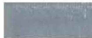
Cutting surface by fiber laser
