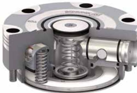
ally, making this process incredibly easy. The actual clamping is done via spring force without any external energy supply; it is form-fit and self-locking. The workpieces remain safely clamped in case of a sudden pressure drop in the air system. A pneumatic system pressure of 6 bar is sufficient to open the clamping modules.
