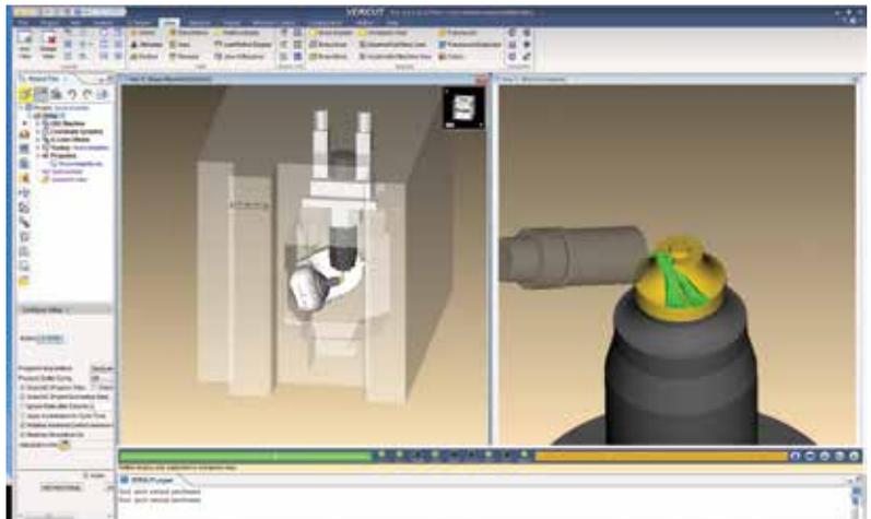
**VERICUT CNC machine simulation, verification and optimization software simulates all types of CNC machining. VERICUT Force™ is a physics-based optimization method that determines the maximum reliable feed rate for a given cutting condition based on the following three factors: maximum chip thickness, maximum allowable feed rate, and force on the cutter. The software operates independently, but can also be integrated with leading CAM systems.**
