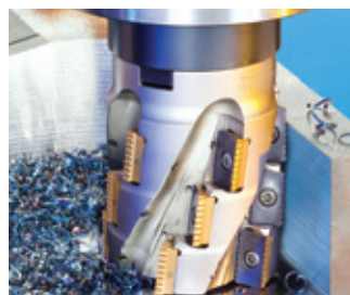
Fig. 3 – Chip-splitting geometry of MILLSHRED indexable milling cutters provides high stable milling and better chip handling.
