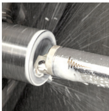
Fig. 2 – In boring, using anti-vibration bars improves performance and reduces power consumption.
