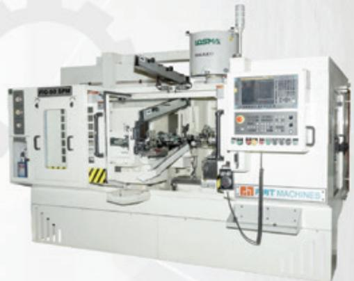
**CNC Internal Grinding**
