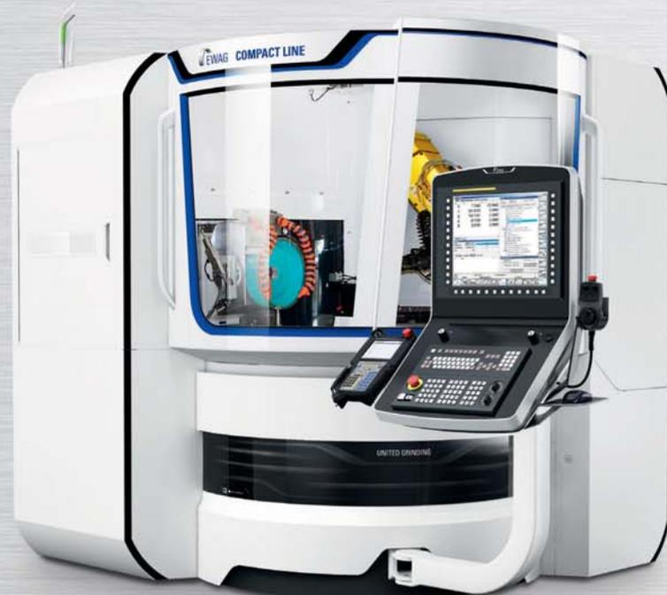
The COMPACT LINE offers maximum grinding performance in the smallest possible space. In production and/or regrinding operations, it grinds indexable inserts made of carbide, cermet, ceramic or PCB/PCD. Depending on the clamping system, the minimum inscribed circle diameter is 4 mm for the pin clamping system and 3 mm for the indexable insert clamping system.
