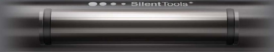
Inside the tool is a pre-tuned damping system that consists of a heavy mass, supported by rubber spring elements. If vibration arise, the kinetic energy will be absorbed by the damping system. This leads to minimized vibration and greatly improved productivity.
