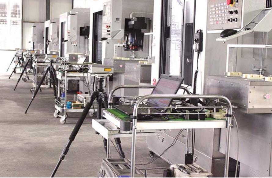
calibrators. Recently Jingdiao has ordered another five XL-80 and XR20-W systems in preparation for its next phase of large batch production and quality control for five-axis machining centres.
