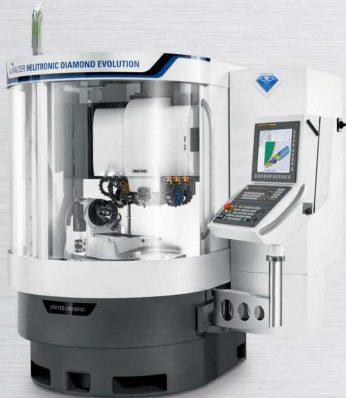
The HELITRONIC DIAMOND EVOLUTION is a high efficient solution within our EDM portfolio for rotary eroding of PCD/CBN tools and grinding of HSS/carbide tools in one single clamping cycle on a minimal footprint. Tool diameters from 1 to 165 mm, tool lengths up to 185 (255) mm, each item can weigh up to 30 kg.
