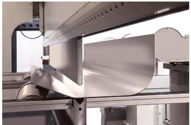
Easy-Form system uses a laser and symmetrical measurement at the front and back of the die to determine the exact value of the angle of the workpiece.
