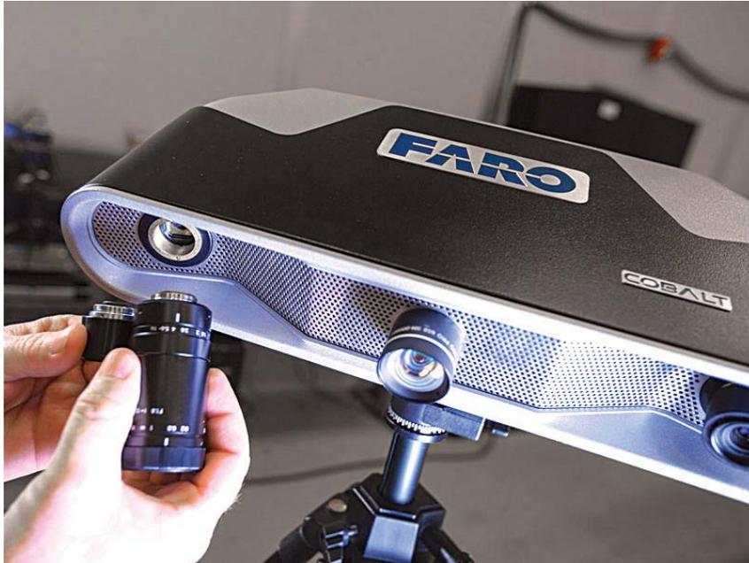
FARO Technologies, Inc., the world's most trusted source for 3D measurement and imaging technology, announces the release of the new FARO Cobalt 3D Imager equipped with a new class of technology and on-board computation capability aimed at improving productivity and operations in the manufacturing sector. The Cobalt 3D Imager is an automated, non-contact variable field coordinate measuring sensor that is easily deployed within manual or automated manufacturing workflows.
