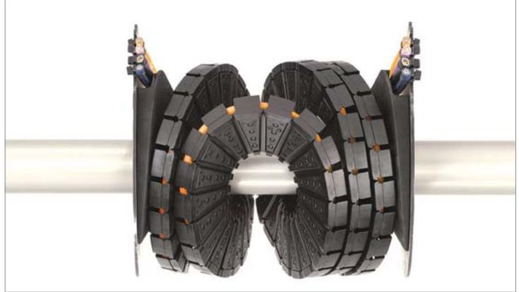
The igus twisterband is used in the e-spool: Thus rotations can be implemented economically and with low wear and low maintenance in a confined space, while reliably guiding energy, data and media. (Source: igus GmbH)
