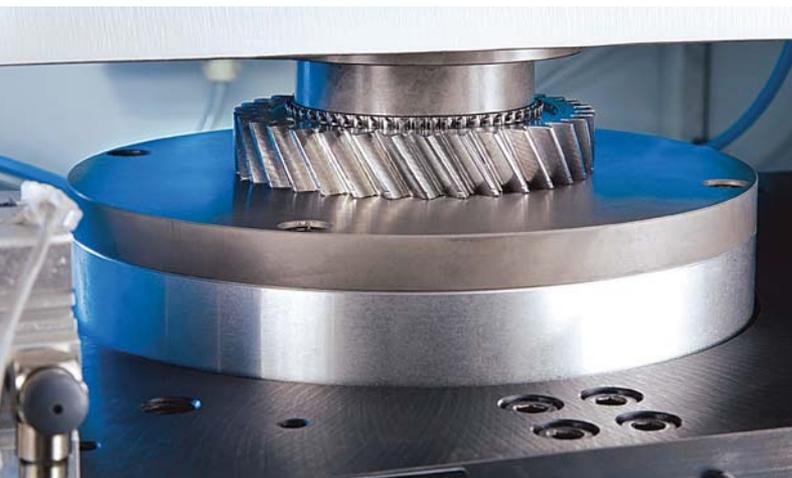
Joining a gear and a synchronous ring on the ELC 160
