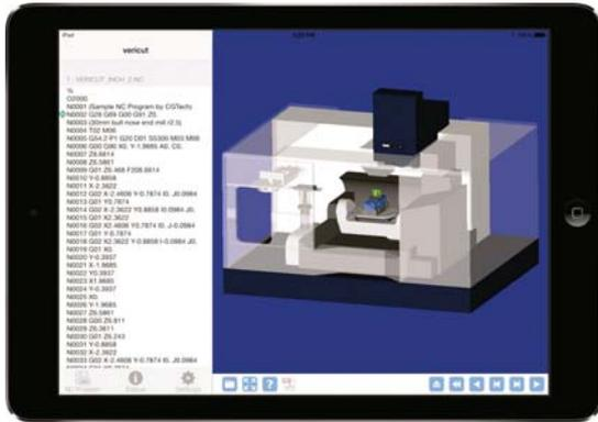
workshop by visually communicating CNC machining processes to the shop floor. It gives machine operators greater confidence when running new or complex machining operations and improves efficiency by quickly referencing current production jobs in meetings, in the factory, during hallway discussions -- virtually anywhere.
