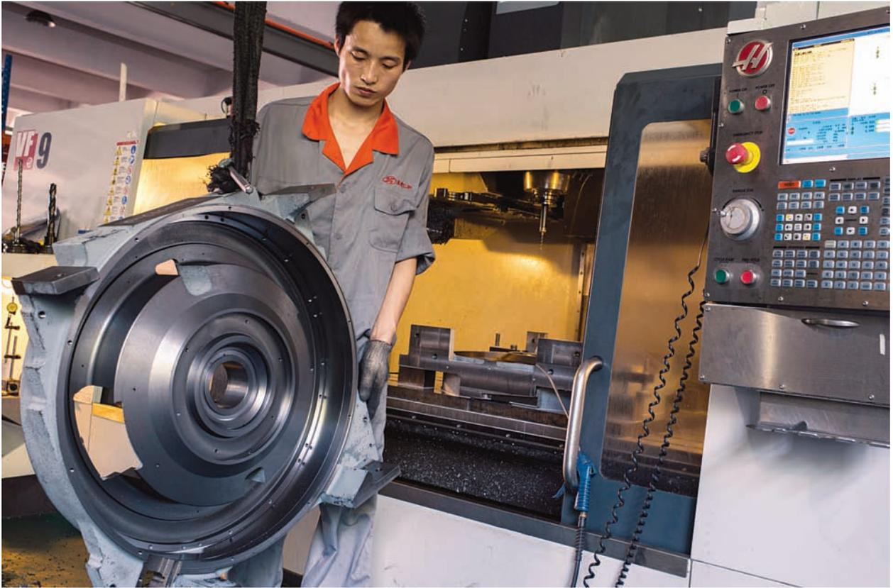
The company's Haas VF-9 makes another, bigger arm for a CNC robot, 2.15m long
