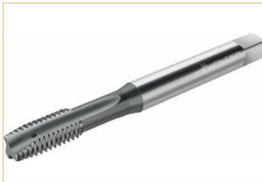
**The Walter Prototyp Prototex® Eco Plus is the multi-talented tool among through-hole taps. A special pre-treatment gives the coating improved adhesion and therefore increases performance. The tool is also available as an option with internal cooling and radial coolant outlet.**
