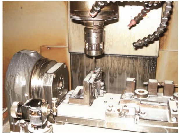
The OMP60 and OTS optical tool setting probe on a machine tool at Associated Tooling.
